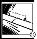
The floor panels have a groove and a tongue or click system, this will enable the floor panels to be fitted into each other mechanically. The only tool that you will need is a hammer, a fine-toothed saw, a folding ruler, a tensioning wire (cord) along the length of the room, a set square, and an installation set consists of a stop block, a stop iron and spacer blocks.
