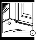
is able to fit the last row, leaving enough space for an expansion gap between the wall and the wood. Although providing a better overall look, continuing boards between adjacent rooms may not be suitable for all room layouts or property types due to excessive movement. What is Underlay A material placed under a wood floor to smooth the subfloor, help cut down airborne noise, protect against damp and/or as a resilient layer under a floating floor.
