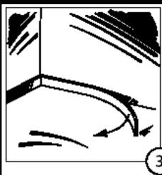
There are several methods of covering the expansion gap once the floor has been installed, depending on the existing site/room and personal preferences or budgetary constraints. Where skirting boards exist, the installers can either remove prior to installation then reinstall above the new flooring or alternatively, the skirting boards can be bottom-trimmed to allow for the new floor to slide underneath. Where skirting boards do not exist, or owners
